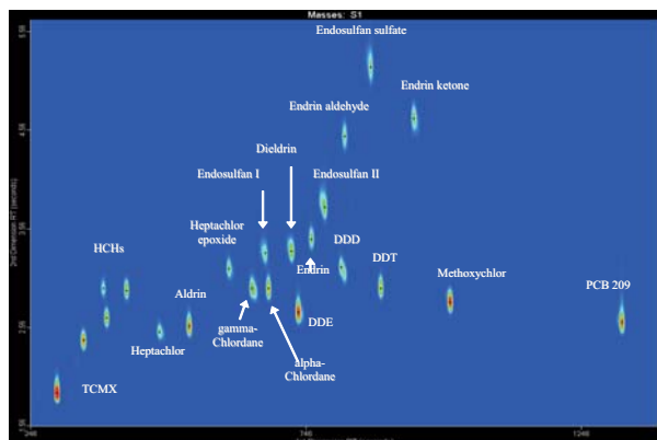
Figure 1. Contour plot (GCxGC chromatogram) of organochlorine pesticide mix. Note the separation of compounds in two dimensions with the Rtx-5 separation (and retention time) on the X-axis, and the Rtx-200 separation occurring along the Y-axis.
